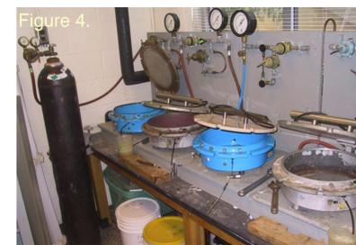
Matric suction is applied to a soil column via positive pressure (Figure 3). High matric suction ( $\geq 1,000$  hPa) is measured with a pressure plate apparatus (Figure 4). The outflow is measured at different matric potentials and plotted as in Figure 1.
