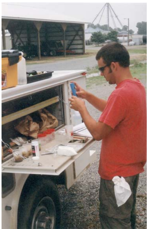
Figure 4. Measurement of pH and soluble salts can be determined quickly in the field.
