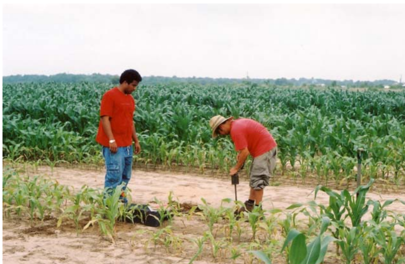
Figure 5. Interns learned to measure soil bulk density and interpret the results. Information derived from bulk density provides insight about physical conditions in the crop rooting zone with respect to the entry and transfer of air, moisture, and heat.
