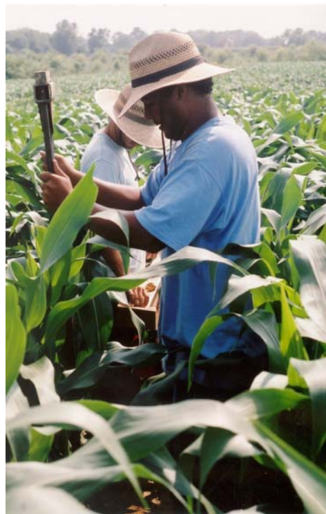
Figure 3. Sampling 45 cm deep using a custom drive hammer and steel tube. Obtaining a representative sample is critical for precision diagnostic inference.
