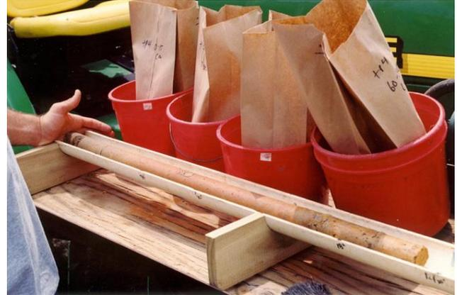
**Figure 7.** View of typical near-undisturbed soil core after extraction from the drive tube. Three cores were collected at each of five transect sampling points and composited.
