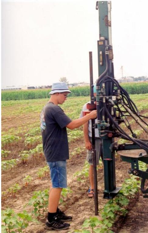
**Figure 6.** Soil coring with the Giddings hydraulic probe. Interns learned to operate the machine as well as extract, clean, section, and composite soil cores.
