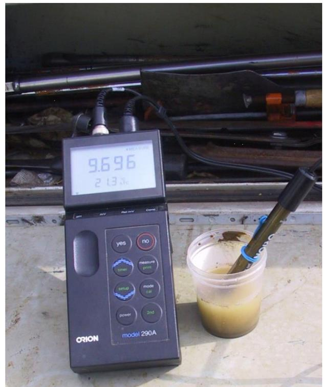
Figure 4. Portable meters like the one shown here are invaluable for on-the-spot soil chemical properties determination.
