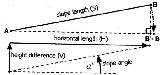
The clinometer is used to measure  $a^\circ$ , the slope angle indicated above. The slope length  $S$  is measured using a tape. Surveyor's tapes that are graduated in 10ths are best for this purpose. Knowing the slope angle and slope length allows one to compute  $H$  horizontal length using the formula:
