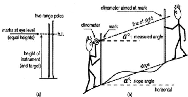
Figure 1. Determination of a slope angle with a clinometer. (a) Two range poles of rods with equal high marks are used for marking a line sight parallel to the slope. (b) The measured angle of this line of sight is equal to the slope angle. Source: *Loedeman, J.H. 2000.*
